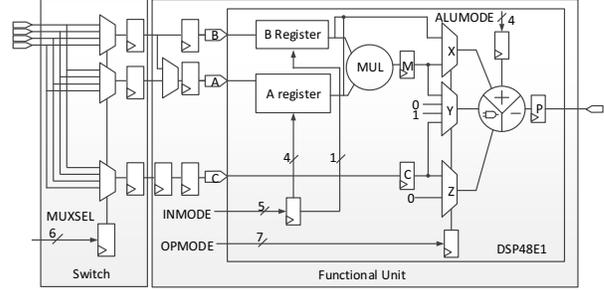
Fig. 4: The 32-bit functional unit and interconnect switch.
