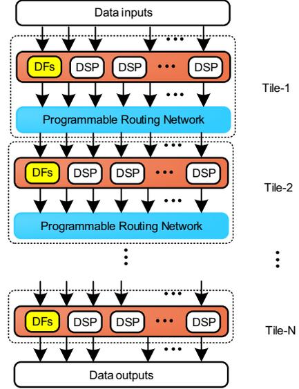
Fig. 1: Block diagram of linear dataflow overlay.
