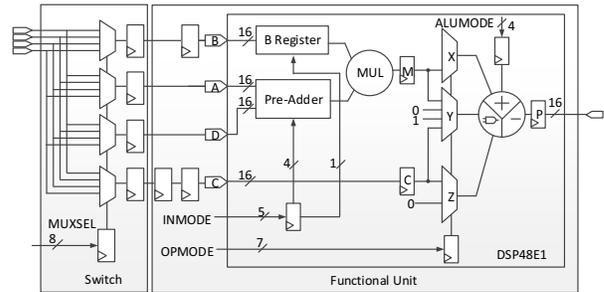
Fig. 5: The 16-bit functional unit and interconnect switch.
