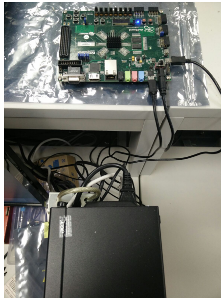
Figure 5.2: The Zedboard-Server Setup
